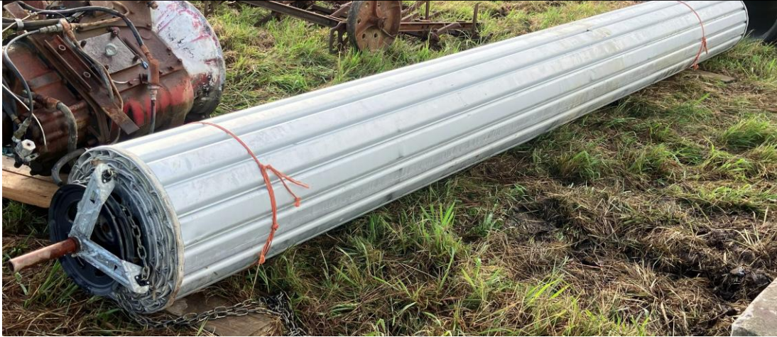
Commercial chain roller door – damaged base
